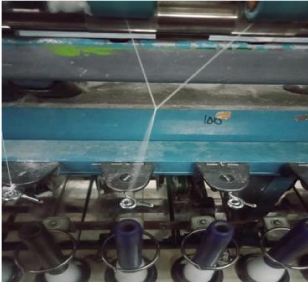
**Gambar 3:** *Defect benang double*
