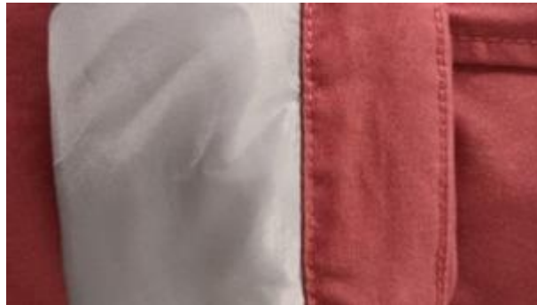
Gambar 2. Defect bubbling pada placket
