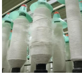
Gambar 1. Roving kotor terkena fly waste
